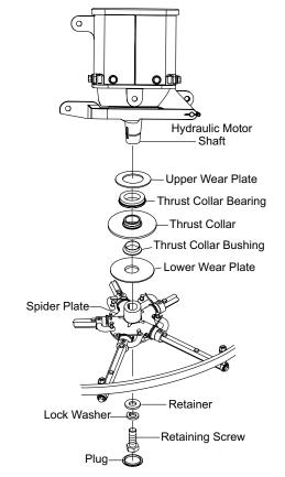
Figure 36. Spider/Gearbox Removal
